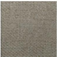
Woven flax fibers as shown here would sandwich a ski core to improve dampening, as well as reduce weight.
